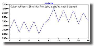
Use LTspice to zero in on worst-case performance by exploring the tolerance limits of components. Here, 16 possible parameter combinations of four resistor values – at their tolerance limits – are simulated and graphed. The effects of tolerance are clearly shown.
