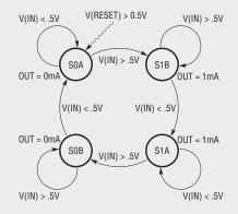
Each state of the state machine is defined using a .state command. The first state listed is the initial state, otherwise the order of the states makes no difference. The name of the state can be anything and the output of the state is defined by a value.
